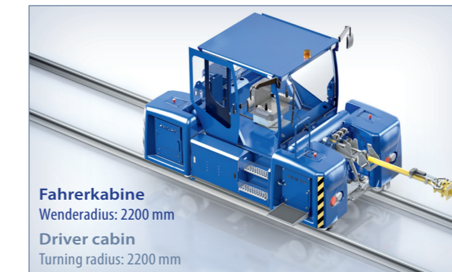
Hybridantrieb Diesel / Elektrisch Hybrid drive Hybrid diesel / electric power
